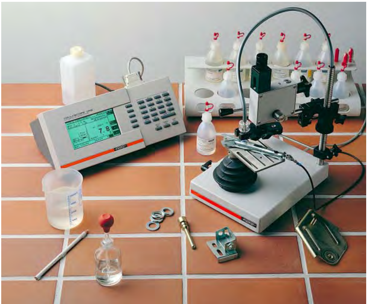
Example for a measurement system with COULOSCOPE® CMS instrument and measurement stand V24
